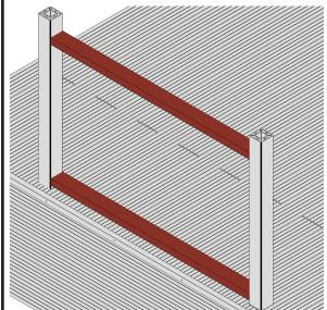
Composite Balustrade Handrail (Part No. ECO09B(S/A/C/G/W) should be used to form both a top handrail, and a bottom rai. These sit between Newel posts and form the frame to hold the spindles.
