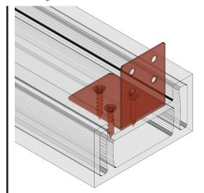
L-Bracket should be positioned to be flush with the end of the Handrail, and fixed - using a good quality 3.5 x 25mm exterior grade screw.
