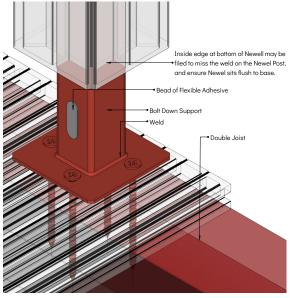
For this method, use exterior grade 7.5mm x 100mm masonry screws to fix the Support through Inside edge at bottom of Newell may be the decking boards and into the filled to miss the weld on the Newel Post, and ensure Newel sits flush to base.
