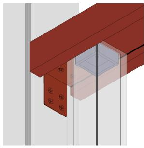
Once the top Handrail is in position, and both the top and bottom Spindle Inserts are fully inserted into the Spindles, the top Handrail should be screwed to the Newel Post using exterior grade 3.5 x 25mm screws.
