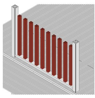
Push spindles onto the lower Spindle Inserts.
