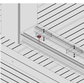
fixed, the bottom Handrail should be screwed down to the substructure through the deck - using a 7.5mm x 100mm masonry Frame Fixing Screw, or similar.
