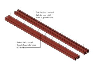
Spindles should be spaced equally between Newel Posts, placed at centres of no more than 99mm.
