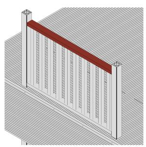
Push top Handrail onto the Spindles.
