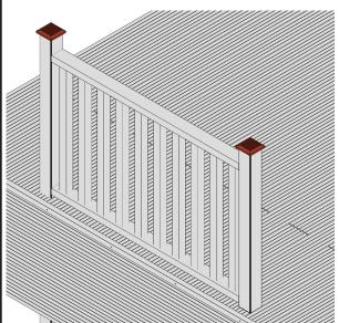
Finally, a Post Cap can be fitted to each Newel - simply push the block on the lower portion of the Post Cap into the top of the recess in the Newel.
