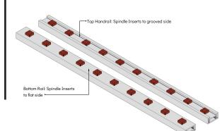
Spindle inserts can now be screwed into the handrail - using a good quality 3.5 x 25mm exterior grade screw. Ensure Spindle inserts are fitted square, as they will determine the orientation of the spindles.
