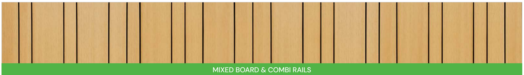
Mixed boards in the following sequence: M, S, L, S, L, M, S, L, S, M, L, M, M, L, M, S, L, S, M, L, S, L, S, M, M, with 6mm shadow gaps, total 24 boards per rail, 8 of each size.
